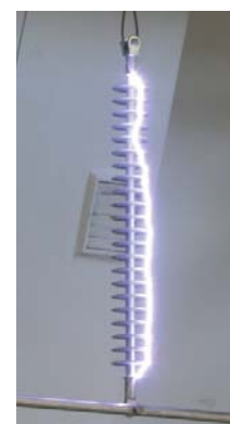
22 Shed Dry LI test
