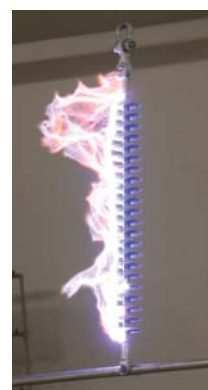
22 Shed Dry AC test
