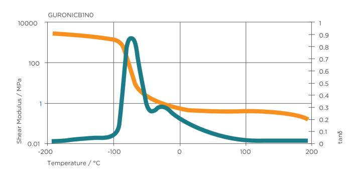
Shear Modulus and damping ( $\tan \delta$ ) dependent on temperature for GURONIC B1NO, used to determine the glass transition temperature according to German industrial standard DIN 53445.
