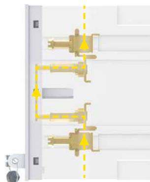
5.2 When lid is put back in place, signals flow again through the socket.
