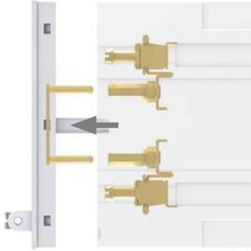
Removing of the lid **opens the circuit**.
