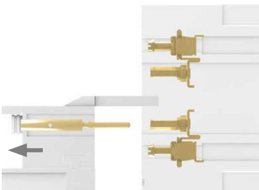
5.1 When the plug is removed, signals are disconnected.
