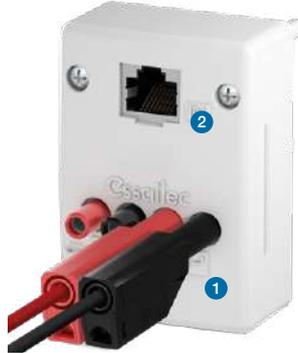
3.2 The ESSAILEC® RJ45 test plug has **built-in dia. 4 (1) and RJ45 test sockets (2)** in order to simplify the test operations. They allow current and voltage **sensors measurement (1)** as well as **injection to the protection relay (2)**.
