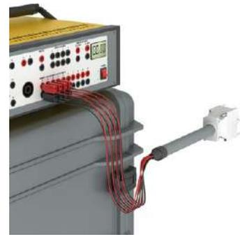
Connect the ESSAILEC® test plug leads to the test set.
